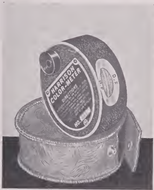
The Harrison Color Meter, designed for use in checking the color balance of all light sources.
