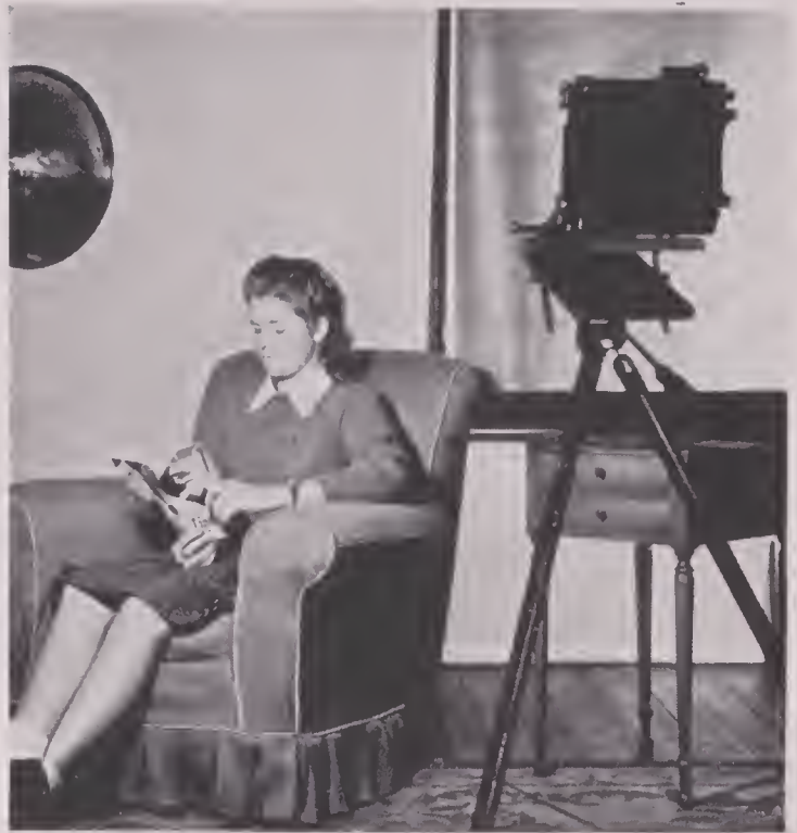
78 Using a reflector with a single photoflood lamp, to open up shadow areas. Reflector set to catch direct light from the photoflood.
