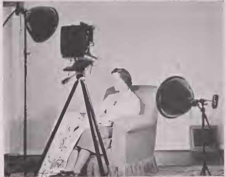
56 This lighting arrangement is identical with that used in Figure 53 except for the addition of background lights. In black and white the effect is "flat," but the contrast range is about right for color.
