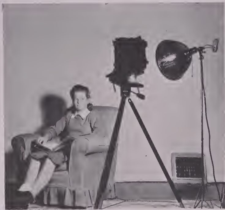
47 The use of a single front light, at or near the camera, creates hard shadows on the "offside" of face and figure, and usually on the background.
