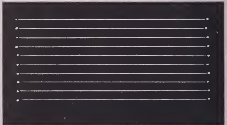
139 Parallel white threads on a black background is another device for checking lateral color correction.
