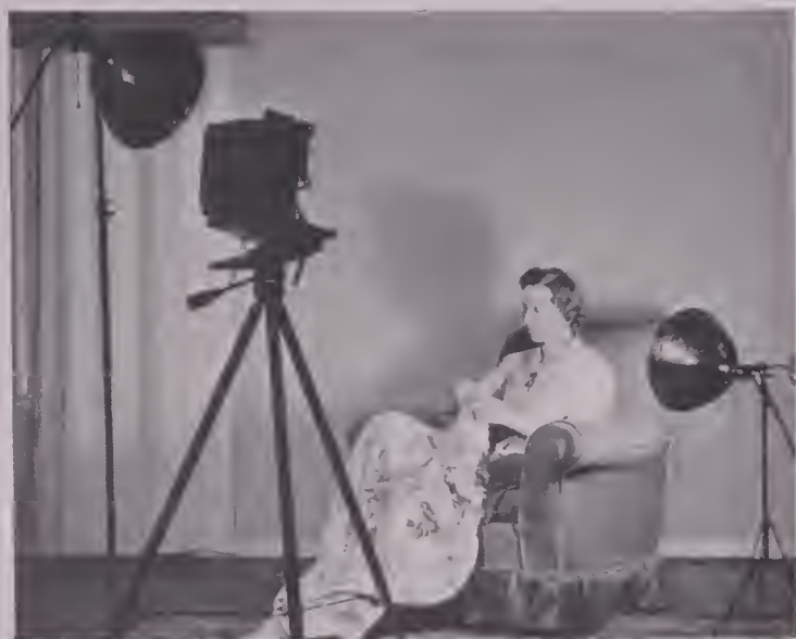
53 Indicated use of a front light at camera, high, and a side light, low, as diagramed in Figure 54.
