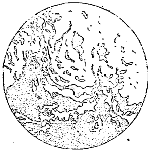
Fig. 2. Showing the tortuous form of a "vermicular" tube (60T) produced by its veining through the matrix. It is to be noted that relics of the latter set in the tube are frequently crescent-shaped, 50 \times .
