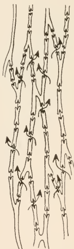
FIG. 56.—Diagram indicating by arrows how the water in the tracheids of pine passes longitudinally from one tracheid to another.
