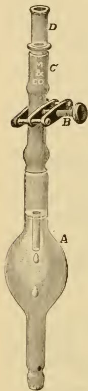
FIG. 128. — COUPLING OF GLASS TO BE PUT IN RUBBER TUBING SO AS TO COUNT THE DROP-RATE, WITH COMPRESSOR TO REGULATE FLOW (Meinecke). (From Hare's "Practical Therapeutics," Lea and Febiger, Publishers.)
