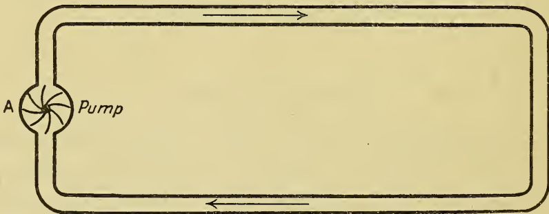
Fig. 2—Water analogy of simple electrical circuit.
