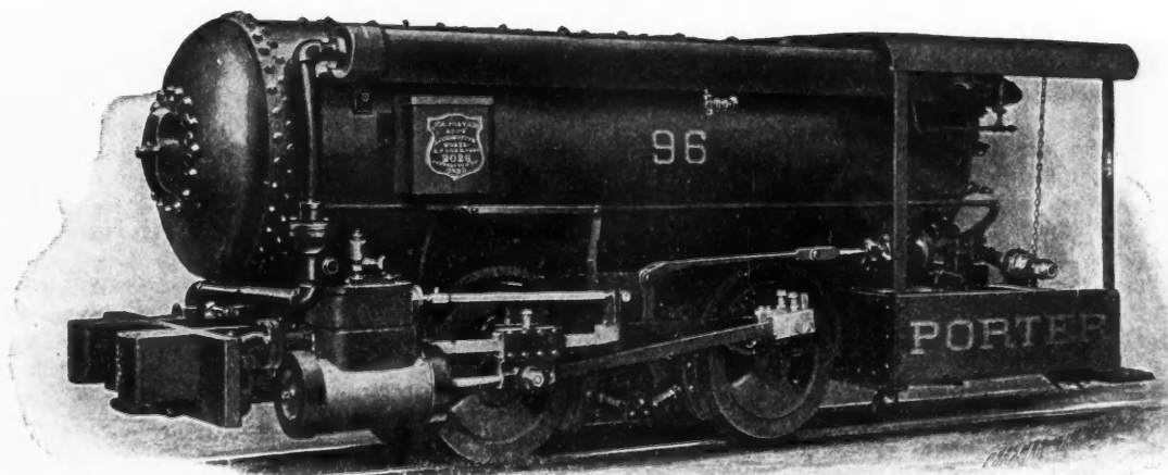
COMPRESSED AIR MINE LOCOMOTIVE. Built by H. K. Porter Company for Commonwealth Iron Company, Cleveland, Ohio.
