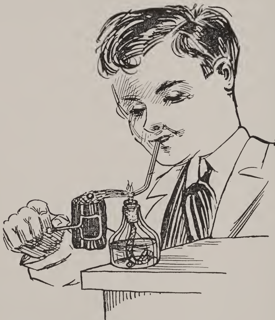
FIG. 126.—How to Heat Antimony with a Blow-Pipe.
