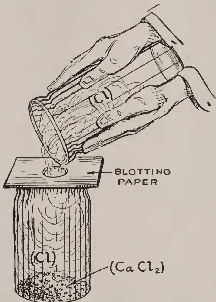
FIG. 96.—Making Some Dry Chlorine Gas.
