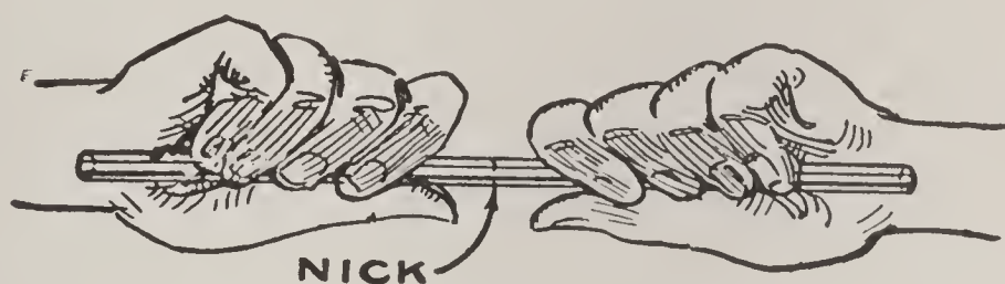
FIG 29.—How to Cut a Glass Tube.
