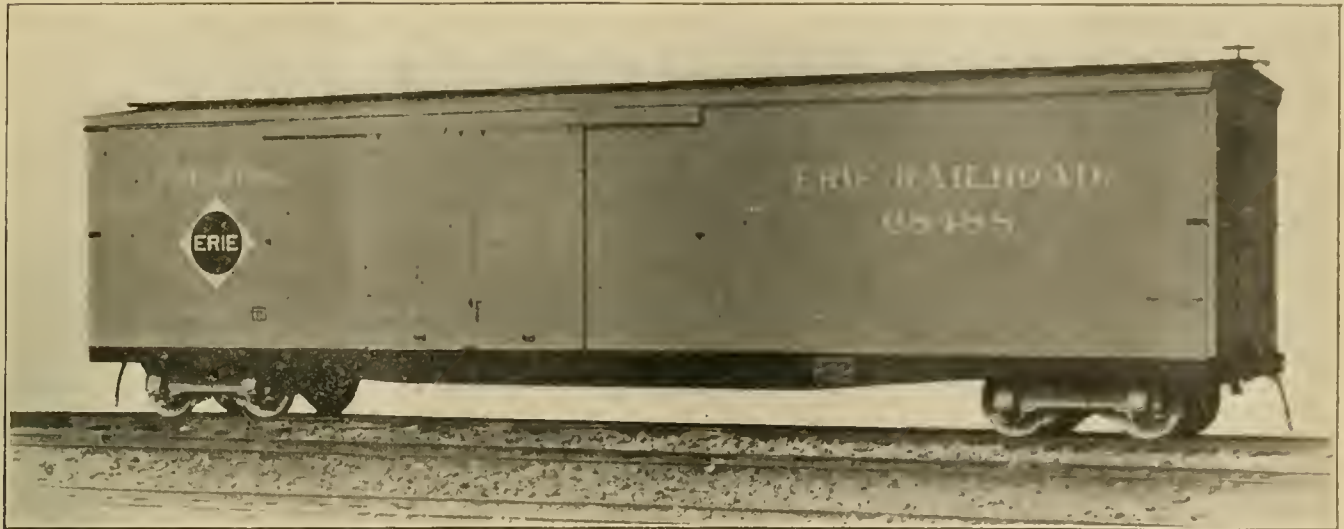
Fifty-Foot Furniture Car, with Steel Underframes—Erie Railroad.
