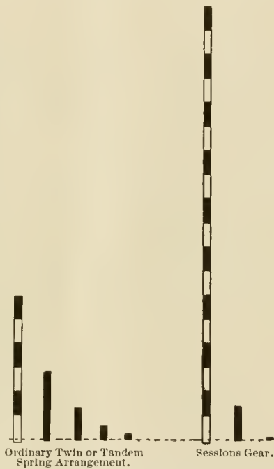
Diagram showing limit of elastic resistance and recoil in drop test of Sessions-Standard Friction Draft Gear, as compared with an ordinary spring arrangement. Two standard M. C. B. springs (3½ x 8 of 12,000 lbs. capacity) used in both cases. Height of broken line shows height of drop and solid lines show recoil of drop.
