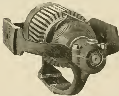
Yoke and Armature, Showing Core with One Coil.
