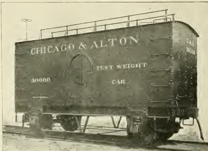
Test Weight Car—Chicago & Alton Railway.
