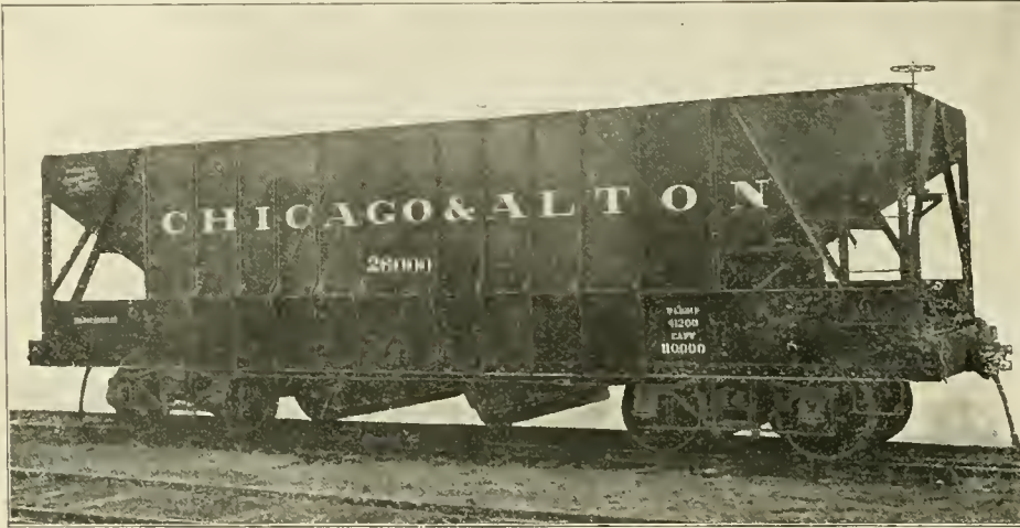
110,000-Pound Capacity Hopper Car—Chicago & Alton Railway.
