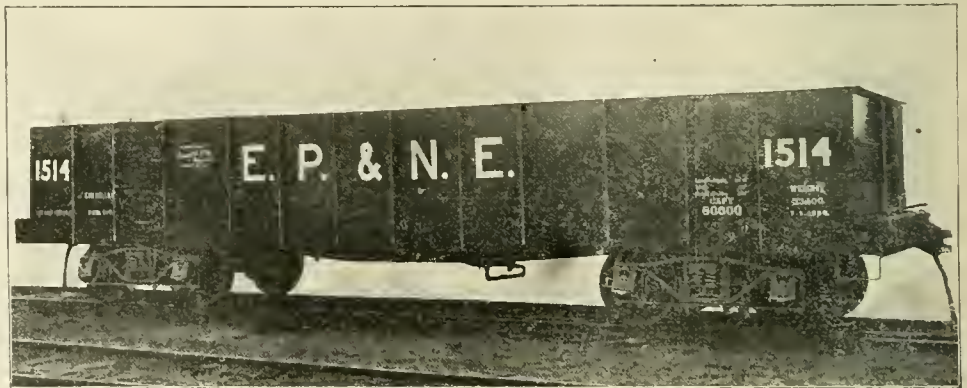
80,000-Pound Drop Bottom Gondola—El Paso & Northeastern Railway.
