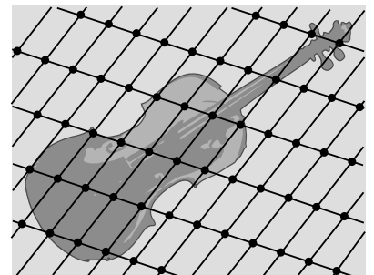
f / Example 3. The area of the viola can be determined by counting the parallelograms formed by the lattice. The area can be determined to any desired precision, by dividing the parallelograms into fractional parts that are as small as necessary.
