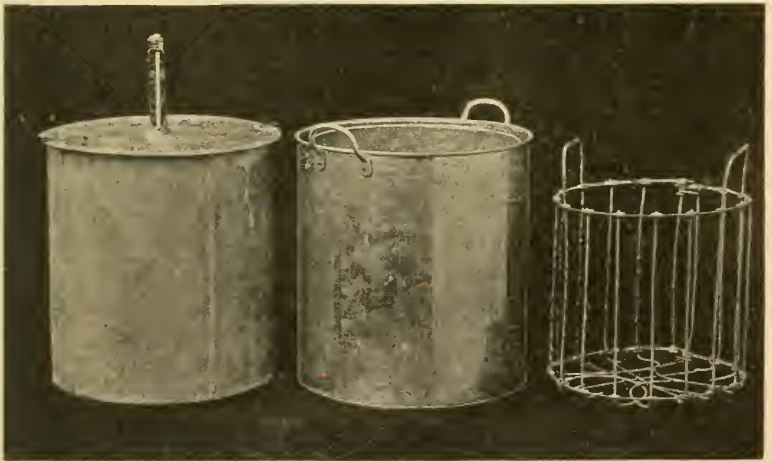
FIG. 63.—Another type known as the water-seal canner requires only a small amount of water and it can be raised quickly to the boiling point with the use of very little fuel. A slight pressure can be secured.
