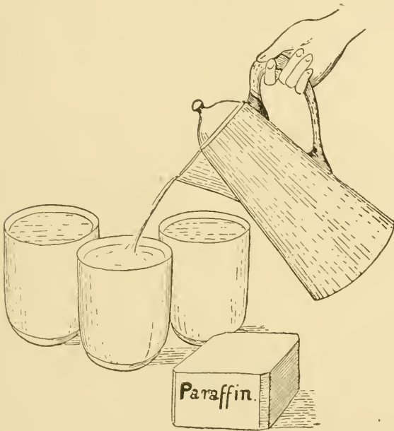
FIG. 105.—A coffee-pot is a convenient utensil for melting and pouring the paraffin.
