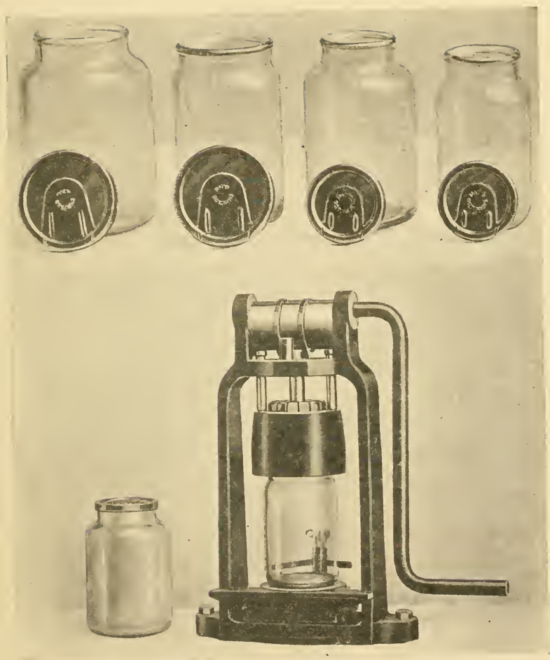
FIG. 38.—Hand sealing machine for glass jars. (Courtesy of American Pure Food Process Co., Baltimore, Md.)
