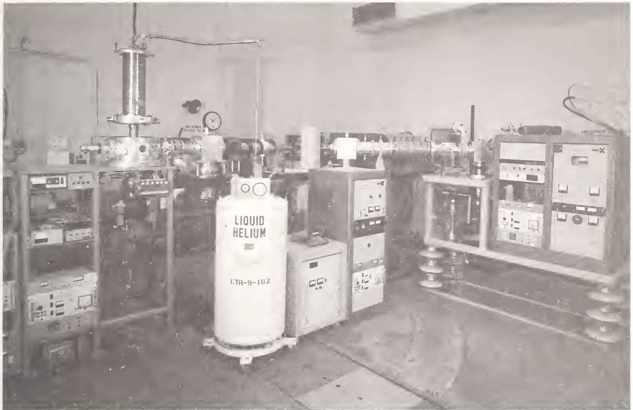
Fig. 6 The Los Alamos Low Energy Fusion Cross Section Experiment. The 120 keV ion source is on the right; the partially disassembled target at the left. The tandem beam line is hidden.
