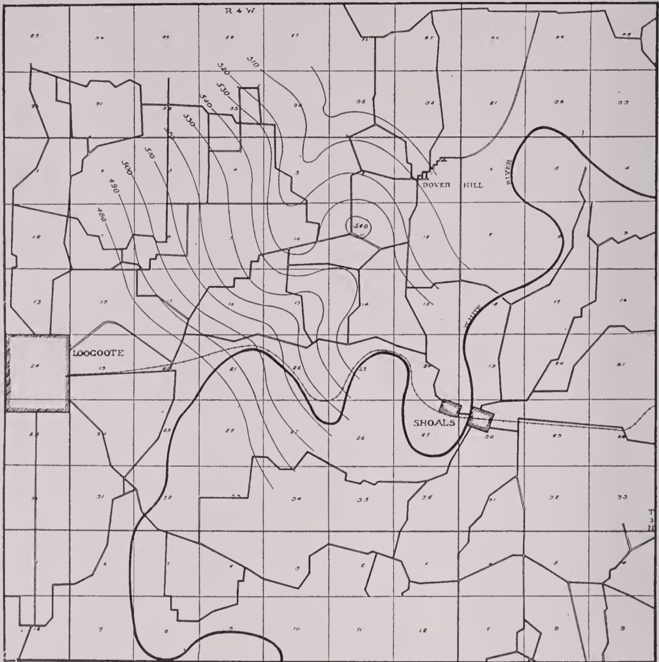
Fig. 47. A structural map of a portion of Martin County showing presence of a terrace. Contours drawn on limestone of Chester series.
