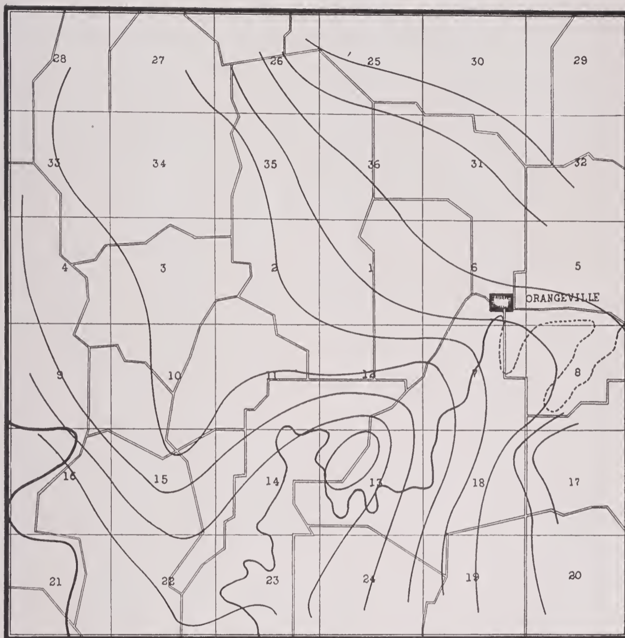
Fig. 51. Map of a portion of Orange County showing structural conditions near Orangeville. Contour lines drawn on Chester limestone. Data secured by C. A. Malott and P. B. Stockdale of field party of 1919.
