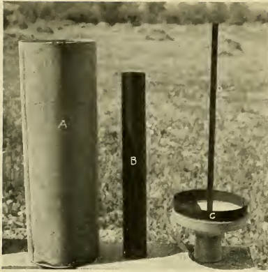
Taken apart, the standard rain-gauge consists of (A) overflow vessel, (B) receiver, (C) funnel, and (D) measuring-stick
