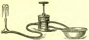
cylinder works smoothly inside another one, and presses down a spiral spring. On rising, it draws up the liquid like a piston, and at the next depression the injection is forced through the tube.
