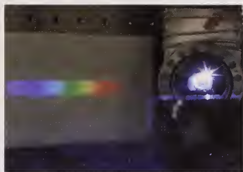
Figure 9. White light from SURF III (right) is reflected by diffraction grating (foreground), to display spectrum on screen.
