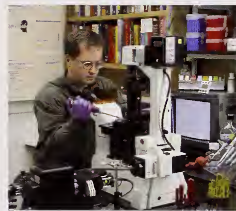
Figure 3. Using a modified microscope, Tom Perkins measures the motion generated by a single enzyme moving along DNA.
