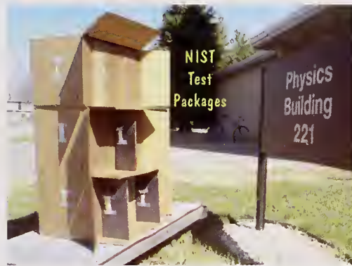
Figure 5. NIST test packages to validate radiation doses needed to decontaminate parcels for U.S. Postal Service.
