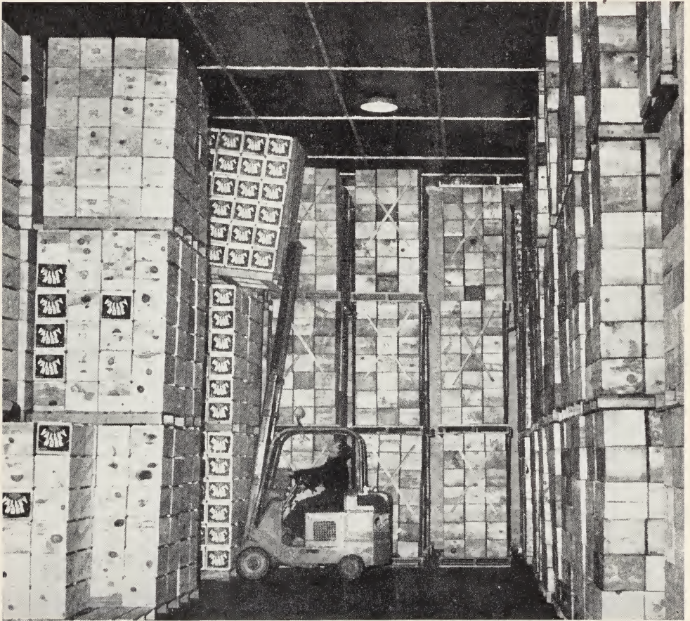
This is typical of pallet loading, using a fork truck for hoisting in a storage warehouse.
