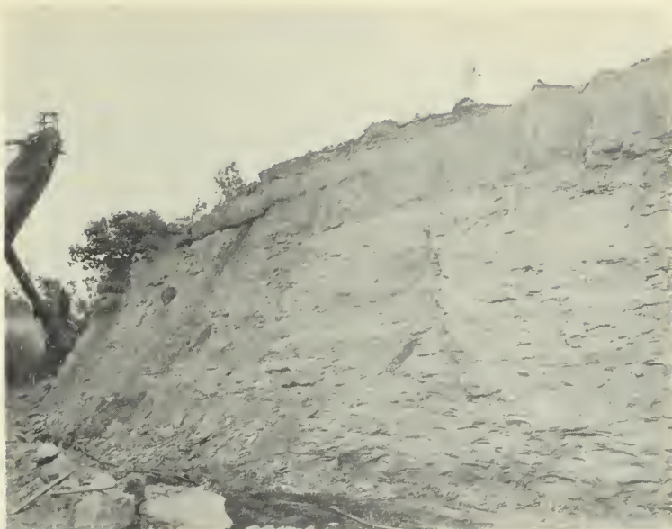
Figure 3.--The overburden of Coal IV usually contains a high proportion of shale and clay. Coal IVa is visible as an intermittent black streak in the upper left corner of this high-wall in Pike County.
