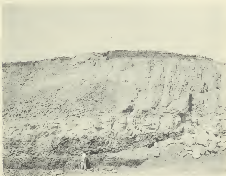
Figure 4.--Massive sandstone and limestone are prominent in the overburden of Coal V. In this Vigo County operation, nearly half of the overburden consisted of calcareous glacial till and boulder clay.
