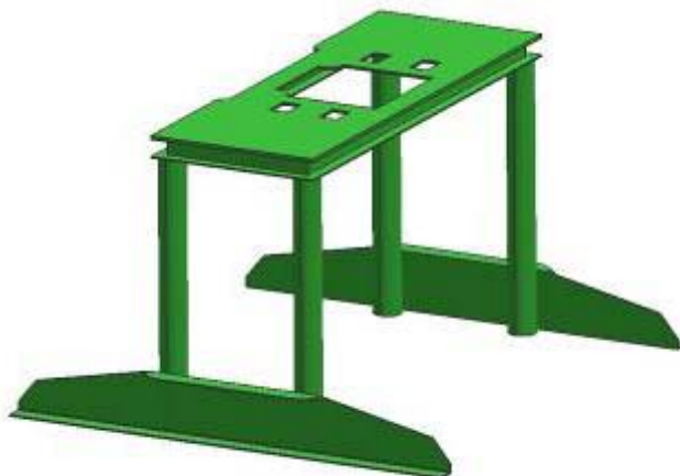
Figure 40. ADaMSat/ABC mate fixture (as of May 2009).
