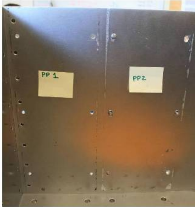
Figure 35. Witness marks on the inside of Wall 1 of NPSCuL-Lite EDU, P2M2 positions 1 and 2
