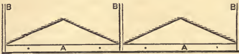
A. Sickle. B. B. B. Guards for supporting the grain, and protecting the sickle.
