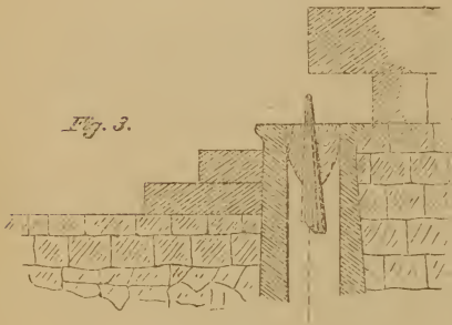
Sketches in plan and section of Egyptian pivot-anchors.
