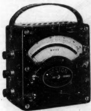
WESTON WATTMETER —Molded Bakelite Case
