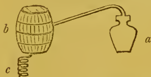
Apparatus for the percolation of alcohol vapour through the dried herb of Indian hemp.
