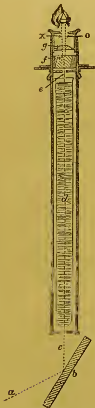
Plan of the Apparatus for showing the circular polarisation of liquids.
