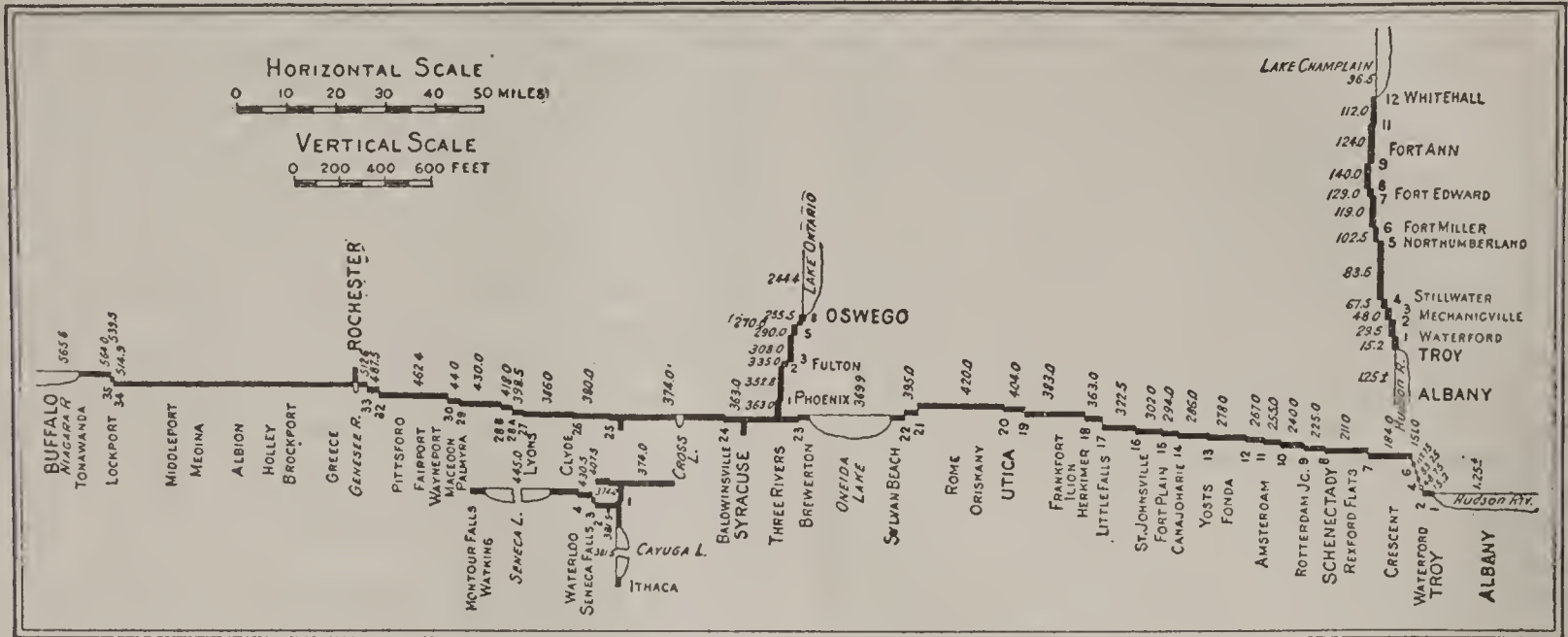
PROFILE OF NEW YORK STATE BARGE CANAL.
