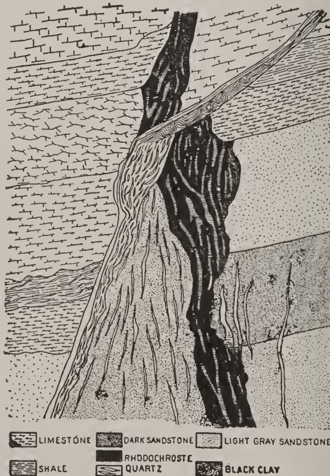
FIG. 4. THE JUMBO VEIN FAULTED BY A CROSS VEIN.
