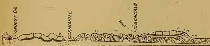
FIG. 11.—Cross section along the south side of Rondout creek through Rosendale. Looking north US., Upper Shaly and Becraft limestones; P., Pentamerus and Tentaculite limestone; C., Cement series; Cl., Clinton and Medina; S., Shawangunk grit; HR., Hudson river shales.
