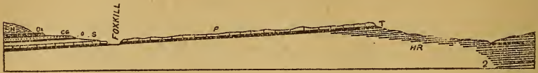
FIG. 5.—Section from near Gallupville across the Helderberg escarpment. H., Hamilton; On., Onondaga limestone; CG, Esopus shale; O., Oriskany; S., Becraft limestone; P., Pentamerus limestone; T., Tentaculite limestone and Salina waterlime; HR., Hudson River formation. Scale, vertical, 3,400 feet to one inch; horizontal, one and three-quarter miles to one inch. Looking west.
