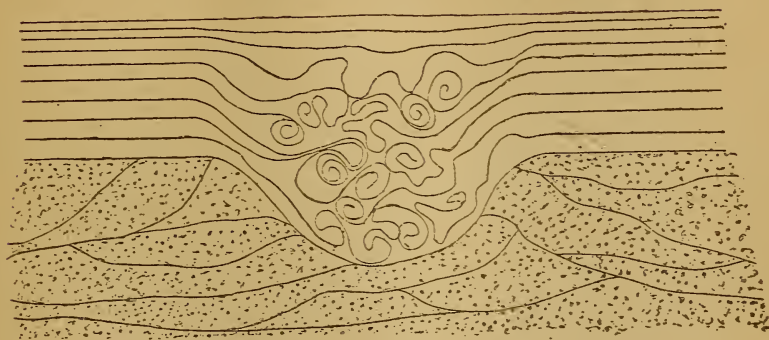
Sand washed from under clay bank causing a flow of the clay.
