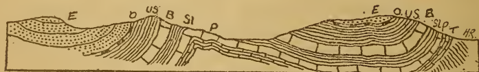
FIG. 4.—Cross section of Rondout Creek valley, just north of Wilbur, N. Y., after Davis. Looking north. E., Esopus shale; O., Oriskany sandstone; US., Upper Shaly limestone; B., Becraft limestone; Sl., Lower Shaly limestone; P., Pentamerus limestone; T., Tentaculite and cement beds; HR., Hudson formation.
