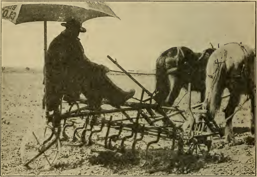
FIG. 5.—Cultivating sugar beets with a 4-row cultivator, which will do twice as much work as a 2-row machine, with practically the same amount of man labor and horse labor.
