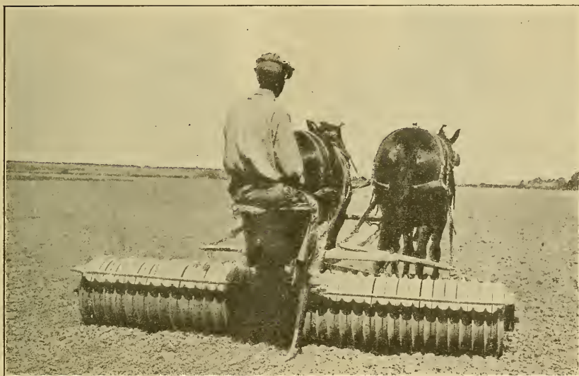
FIG. 4.—A corrugated roller used on beet land. A good type of roller for firming the seed bed.
