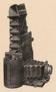
HE 1A Graflex combines all the exclusive Graflex features with film simplicity and convenience. It is equipped with the Graflex Focal Plane Shutter for making exposures from "time" to 1-1000 of a second. The image can be seen right side up, the size it will appear in the negative, up to the instant of exposure.
