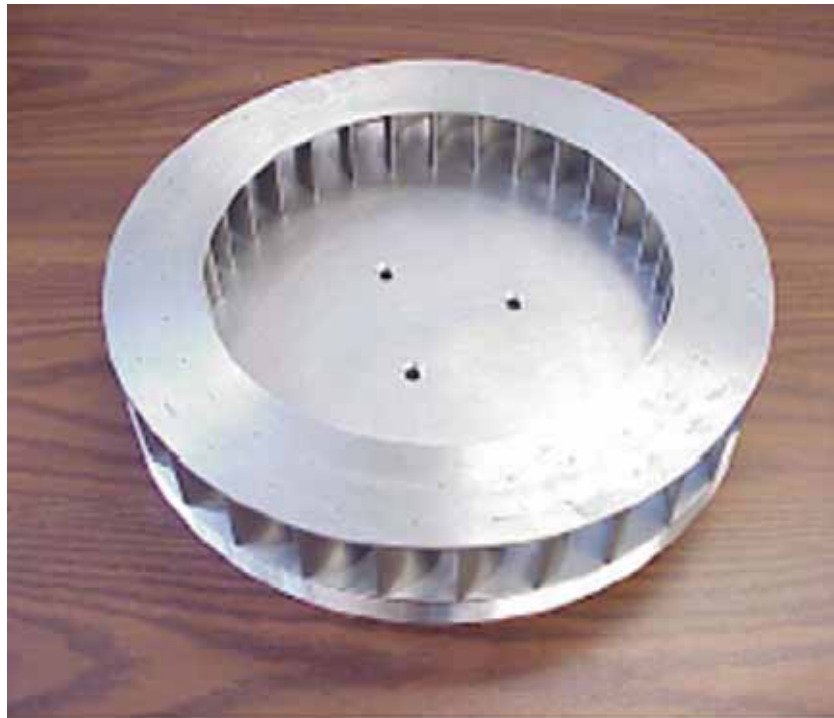
Figure 2. Twelve inch by one and one half inch crossflow fan tested at NPS TPL (From Ref. 3)
