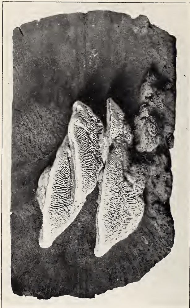
DAEDALEA QUERCINA ON OAK RAILROAD TIE. PORES ON THE UNDERSIDE. (Photograph by Dr. Herman von Sehrenk.)
