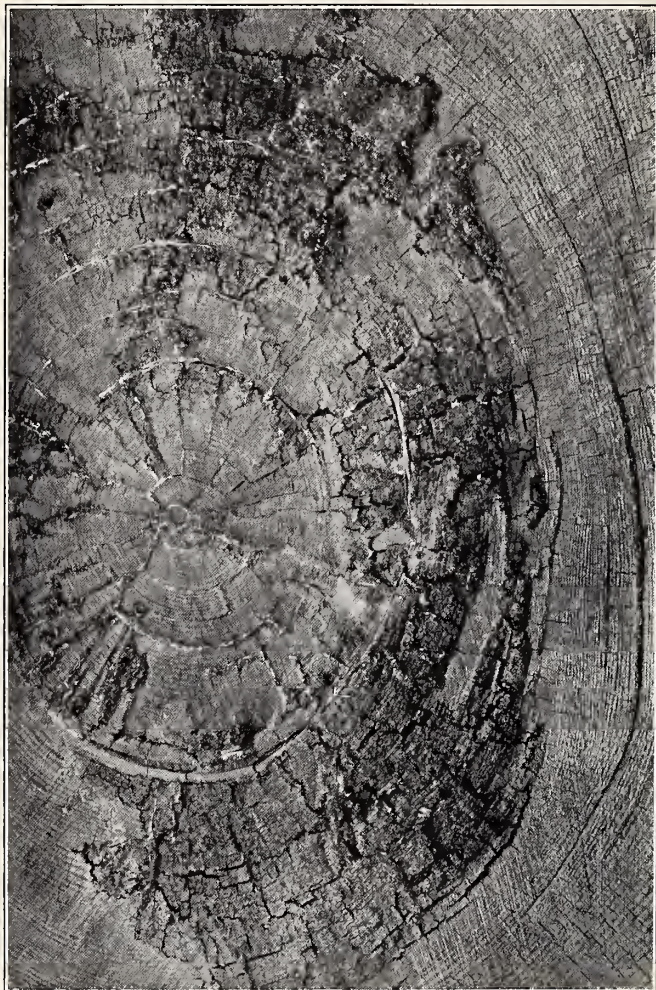
CHALKY QUININE FUNGUS ( FOMES LARICIS ) IN LODGEPOLE PINE. TYPICAL ROT OF THE HEARTWOOD WITH FELTS OF WHITE MYCELIUM IN THE CRACKS.
