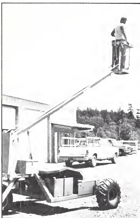
Richard Jaeger, labor supervisor at the J.E. Schroeder Seed Orchard near Woodburn, Oregon, demonstrates the "orchard ape," a lift that extends 20 feet in height and can be operated by one person to help with several operations, including pollinating flowers and picking cones. The orchard is operated by the Oregon Department of Forestry.
