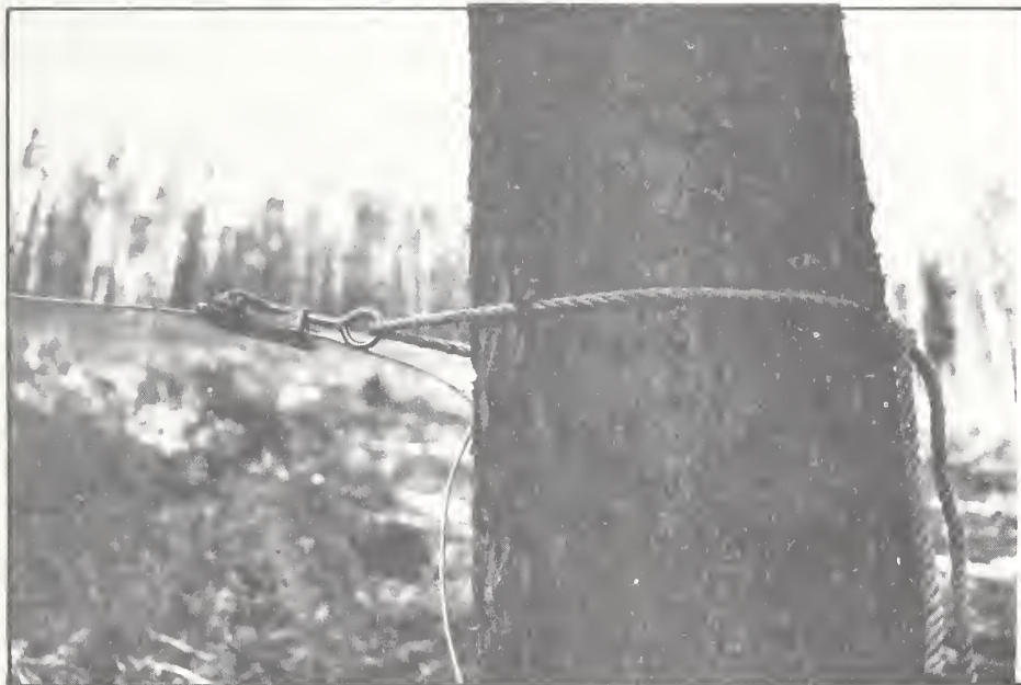
One end of the skyline is attached with a come-along that keeps the wire taut (top). The other end is secured using a nylon rope and quick release wire grip (bottom).
