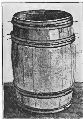
Fig. 45. Nailing the quarter hoops. The chine hoops are not nailed until head is in place.
