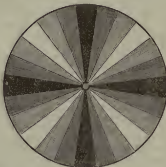
FIG. 8.—Mica disk of twenty-four rays, showing black cross in the dark field.
