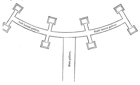
tamp, beginning at the termination of the main gallery, say one hundred feet, leaving all the air space in the side galleries. Run out some five or six fuzes and two wires, to render the ignition of the charge certain. "I propose to put in each of the eight magazines from 1,200 to 1,400 pounds of powder
