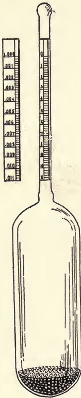
FIG. 24.—Salinometer. A glass bulb weighted with shot and carrying a scale for measuring the amount of salt in seawater.
