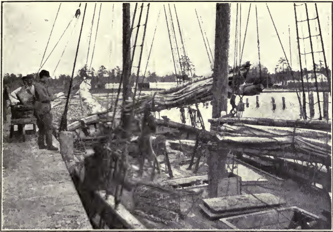
FIG. 31. A North Carolina dredging schooner, showing dredge and hand-windlass. From Dr. Caswell Grave in U. S. F. C. Report.
