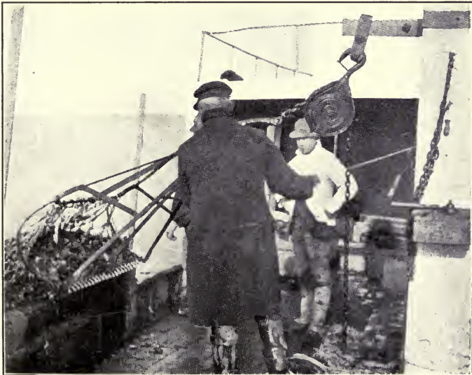
FIG. 32. Drawing a more modern dredge by steam power on the New York oyster grounds. From a Report of the N. Y. Forest, Fish and Game Commission.
