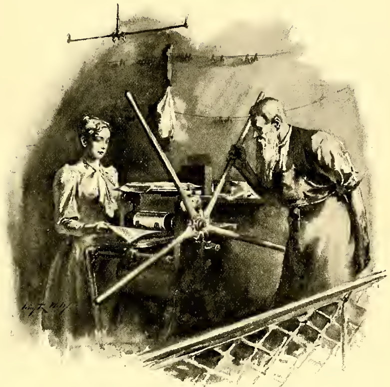
PRINTING SHEETS OF BILLS ON ONE OF THE HAND-PRESSES.
