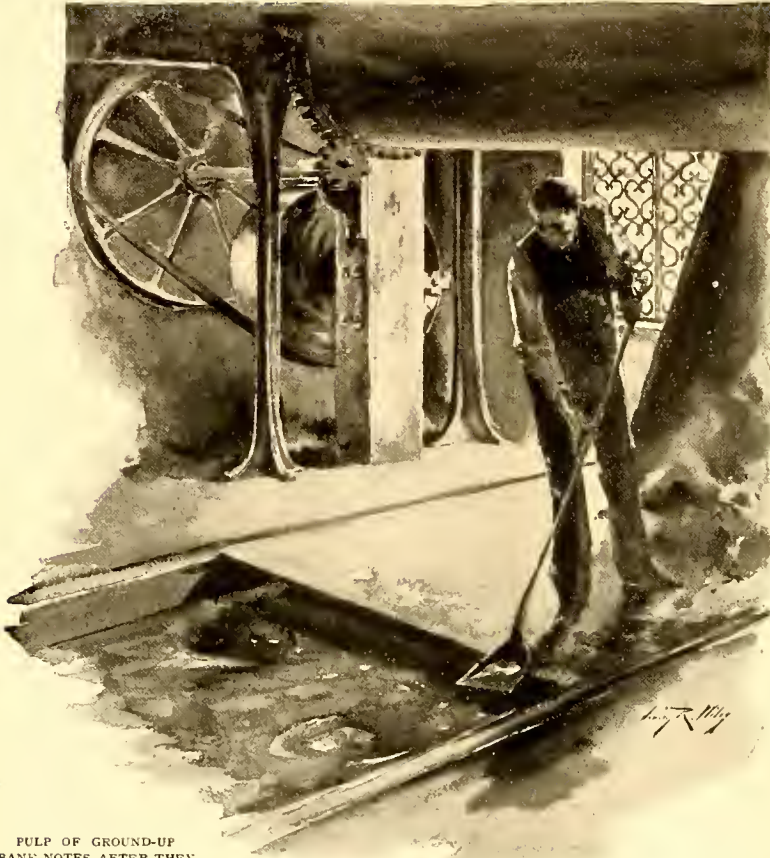
PULP OF GROUND-UP BANK-NOTES AFTER THEY HAVE BEEN DESTROYED BY THE MACERATOR.
