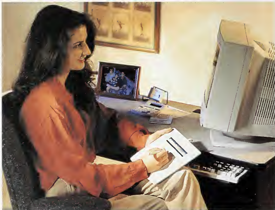
A computer user entering information into her PC with a pad and stylus. Company software in the PC converts the data from the pad into letters and words.
