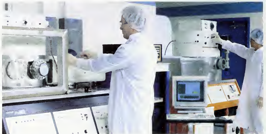
The clean room at Nonvolatile Electronics in which GMR sensors and other devices are fabricated.
