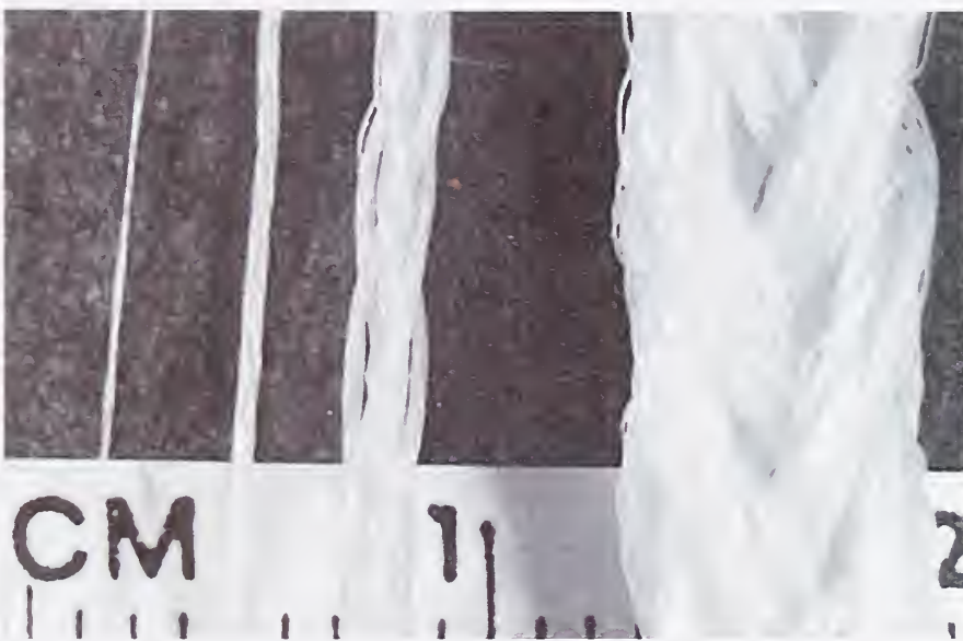
Collagen fiber and braided structures from collagen fiber: (a) single collagen fiber, (b) 8-ply collagen fiber braid, (c) 64-ply collagen fiber braid, (d) 512-ply collagen fiber braid.
