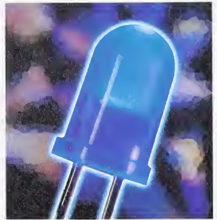
The low-cost blue light emitting diode (LED) produced with new silicon carbide crystal technology.
