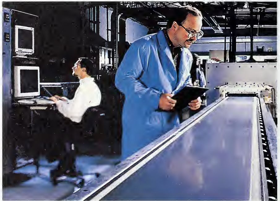
A large area solar grade silicon sheet emerging from a silicon growth reactor which incorporates new ATP-funded technology.
