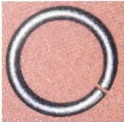
A ceramic toroid form, coated with thick film HTS material, designed to resonate at a specific frequency.
