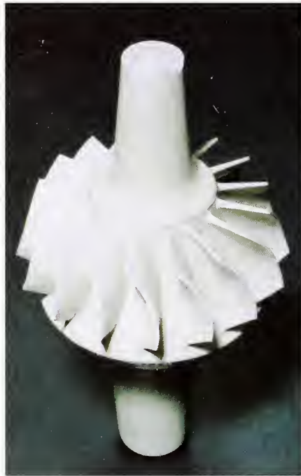
A 16-blade silicon nitride turbine wheel for use in small turbogenerators.
