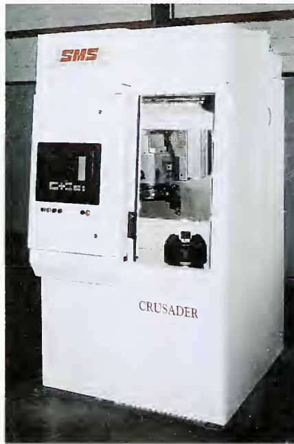
A new high-precision vertical lathe which incorporates the new thermal-error compensation technology, first delivered to customers in 1998.
