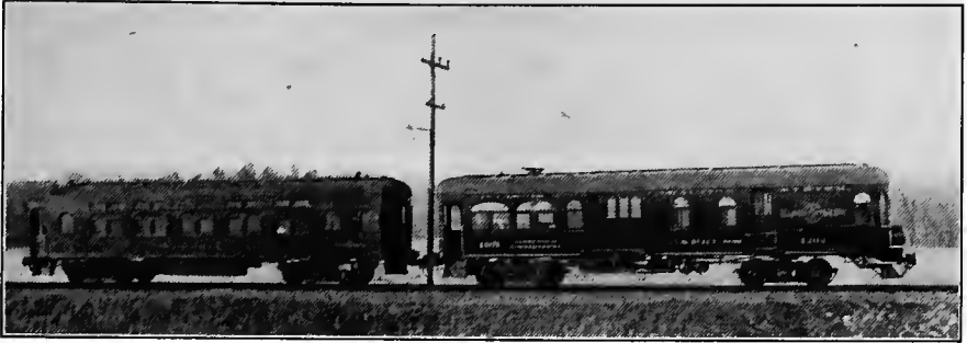
FIG. 102.—Combination train on Illinois Traction System consisting of baggage and passenger motor car and sleeping car as trailer.
