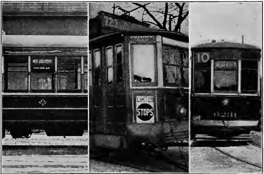
FIG. 107.—Side route sign on end entrance car in Buffalo. Limited stop sign in Boston. Vestibule route sign in Buffalo.
