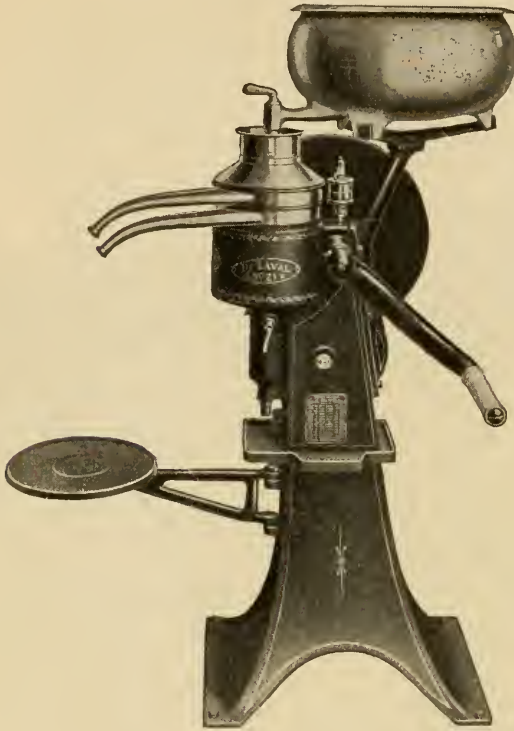
Fig. 4. Making cream by centrifugal method or separator
