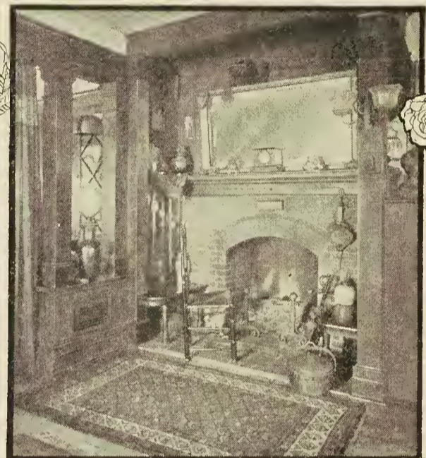
The angle-nook in the reception hall is cosily protected from draughts. This centring of the one chimney diffuses the heat economically through all the rooms.
