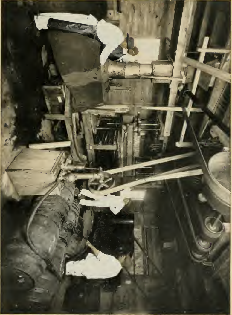
CIDER-PRESS DRIVEN BY A GASOLINE ENGINE. The juice as it runs out is immediately pumped into barrels.
