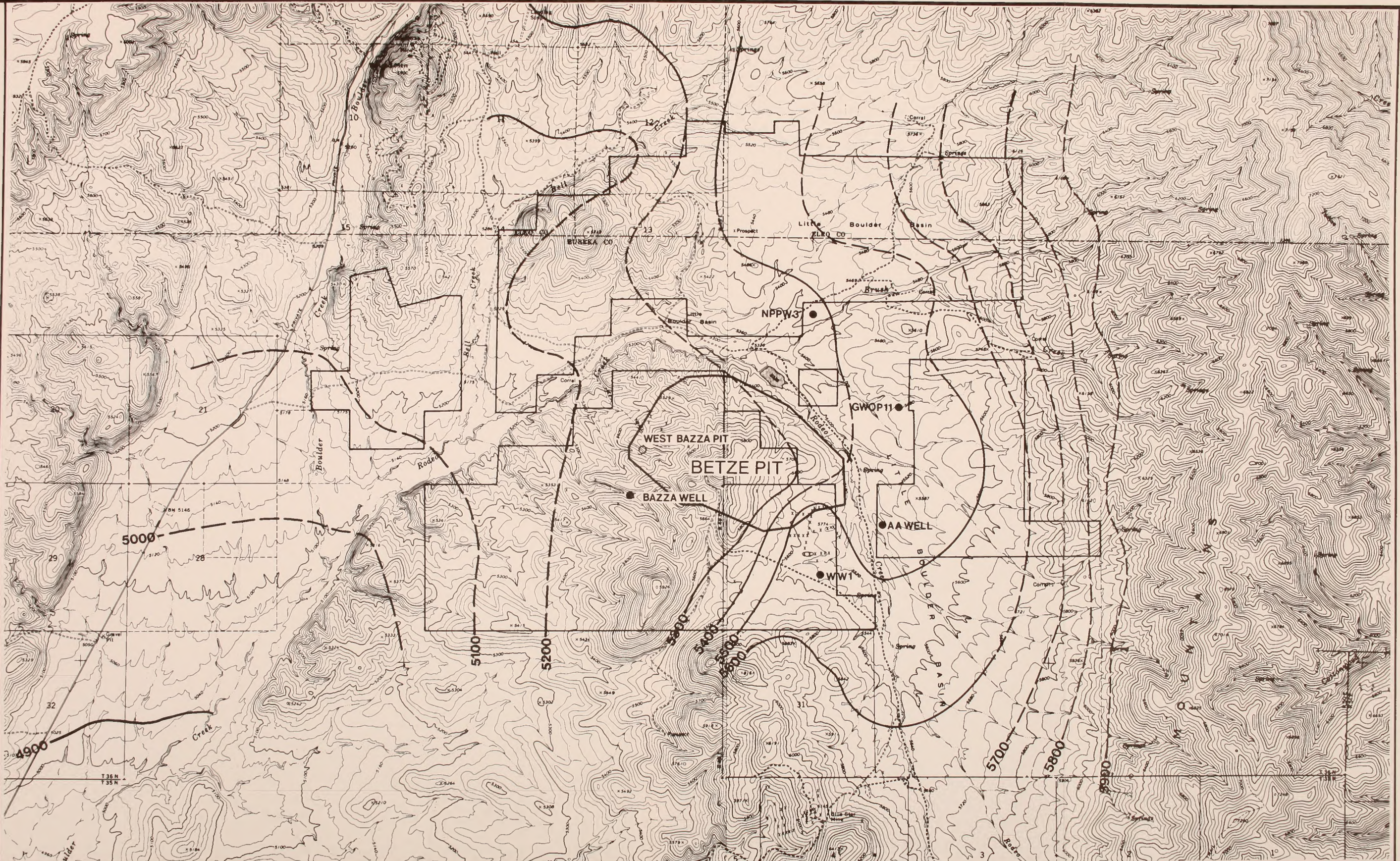
Figure 4-12. Pre-Dewatering Groundwater Elevations and Well Locations
