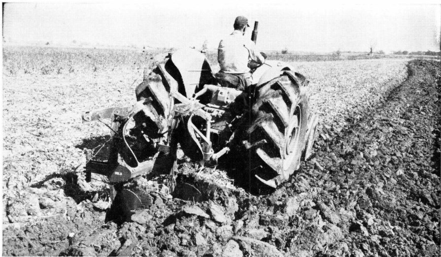
Plowing under the waste cotton and shredded stalks. Very few pink bollworms survive the winter when buried in wet soil by this practice.
