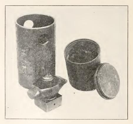
Fig. 1. Photograph of the parts of the autoclave
