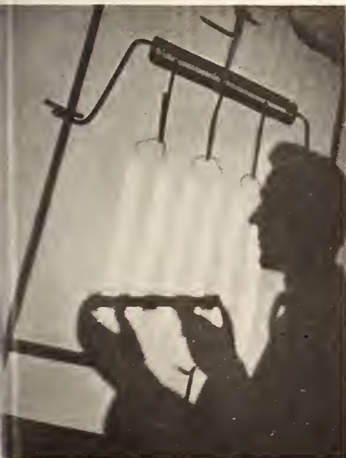
Light magnified — silhouette of a Westinghouse engi- neer measuring the expansion of the filaments of a 100-watt projection lamp. The burning filaments are magnified 35 times for such studies.
