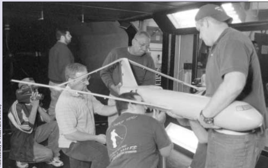
Photo courtesy of Texas A&M University Texas A&M University is one of the few not experiencing a decrease in engineering enrollments. Shown here, A&M aerospace students prepare an airplane model for wind tunnel testing.
