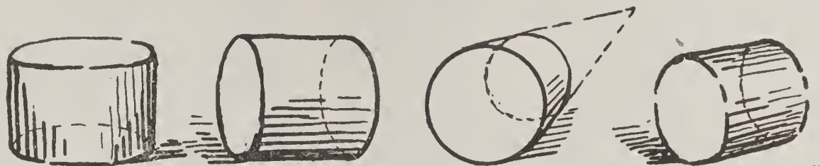
The Vertical cylinder. The Horizontal cylinder. The Receding cylinder. The Oblique cylinder.
