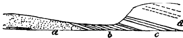
FIG. 39.—SECTION ACROSS THE UPPER SECONDARY ROCKS OF ENGLAND. a. Chalk. b. Weald clay. c. Greensands and Gault. d. Hastings sand.
