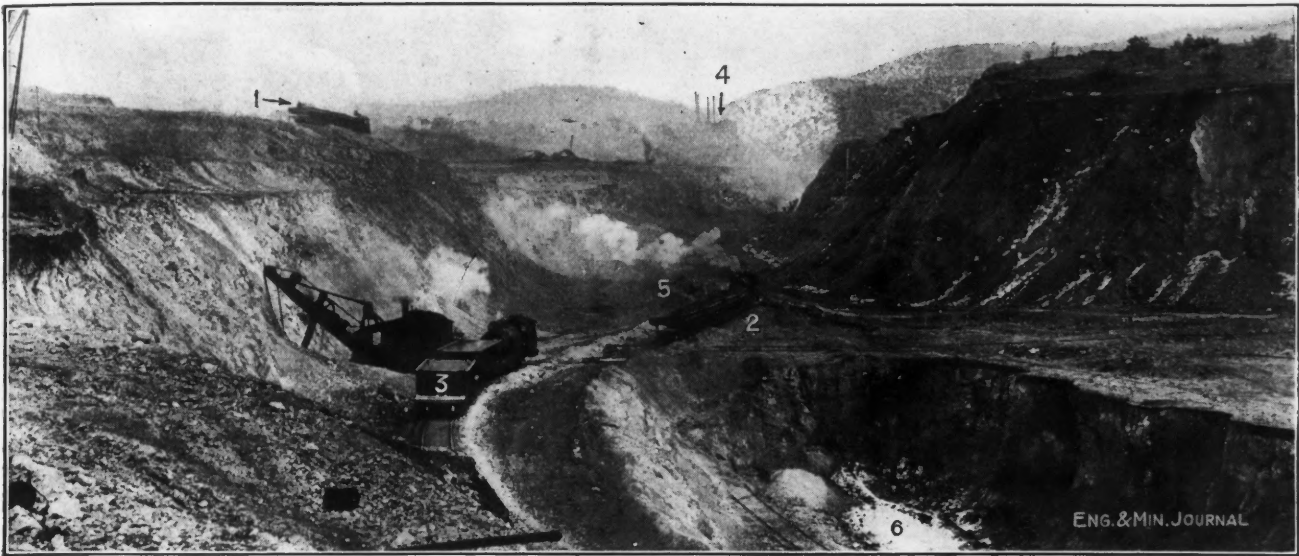
VIEW FROM ORE PILE NO. 1, LOOKING EAST THROUGH NORTHEAST OREBODY PIT FROM WEST SIDE OF WORKS 1, Waste train of 12-yd. cars; 2, waste train; 3, ore train of 50-ton cars; 4, Santa Rita hoist house; 5, 6300 bench connecting northeast and west orebodies; 6, 6250 bench, west orebody.
