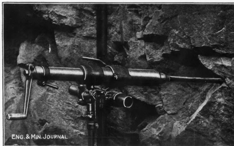
FIG. 1. SIDE VIEW OF MOUNTED MODEL. NOTE CLAMP AND ROTATING HANDLE
