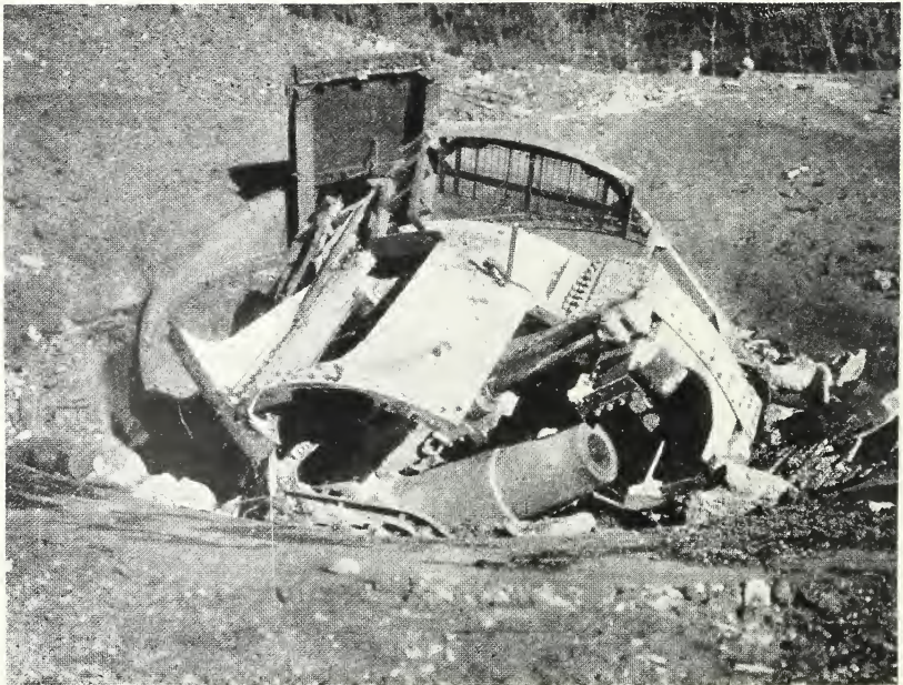
German twenty-eight centimetre howitzer and turret at Tsing-Tau destroyed by the Japanese gun fire.
