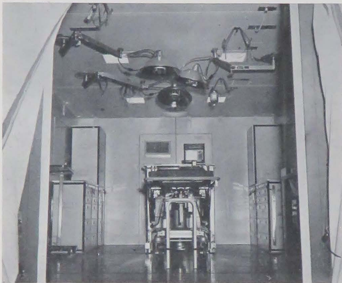
Interior of the MUST unit resembles any other operating room. All equipment is contained and carried in the center section when the unit is contracted when being moved from place to place.
